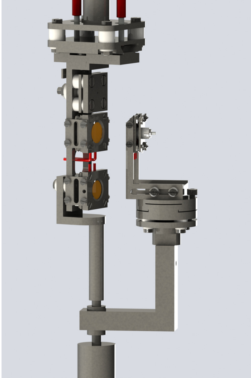
Figure 6: 3D model of target and catcher holder. A Faraday cup (FC), the primary QCM and the pellet are mounted on the sample holder from top to bottom. The heating wires of the samples are represented in red. The insertion tube as well as the catcher holder's rod can be seen at the bottom of the constellation.
